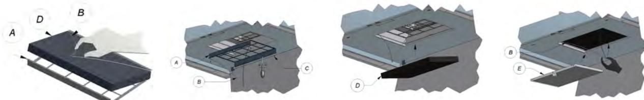
**Programming a saturated carbon filter (Caution: carry out the programming with the motor disabled):**
